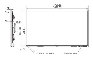
**86"**  $\begin{vmatrix} 1955^{W} \times 1162.5^{H} \times 126^{D} \text{ mm} / 77 \times 45.8 \times 5 \text{ inch } 58 \text{ kg} / 127.89 \text{ lbs} \end{vmatrix}$
